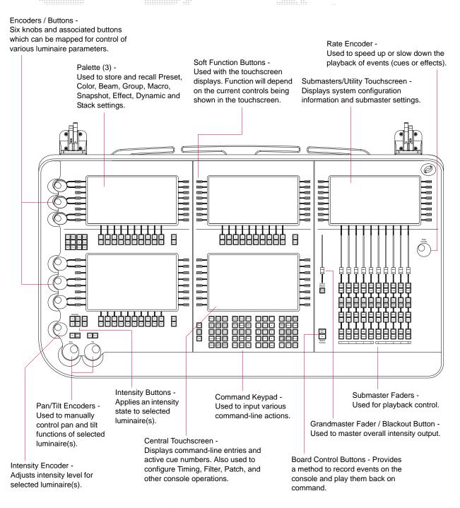
Figure 2: V676 Front Panel Layout
