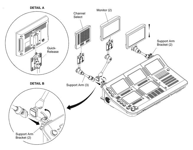
Figure 5: Installing Channel Select Panel and Monitors on V676 Console (Optional)
