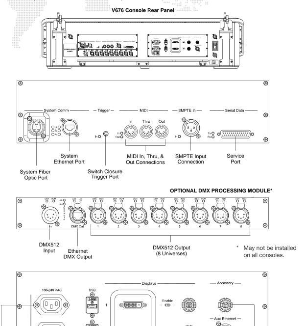
Figure 8: V676 Console Rear Panel Connections
