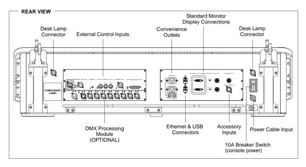
Figure 3: V676 Console Front and Rear Panels
