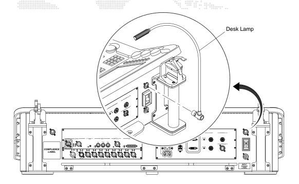
Figure 7: Installing Desk Lamps
