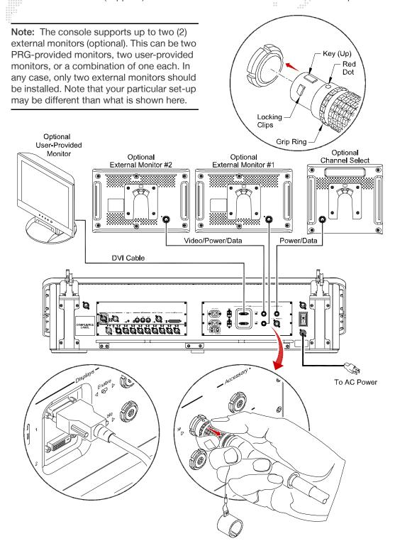
Figure 6: Connecting Components to V676 Console
