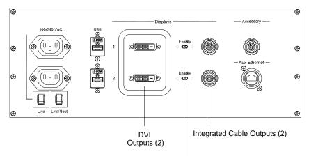
Toggle Switches (2) -Toggles between DVI output or Integrated Cable output
