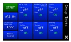
**Group Tests Screen** - Allows multiple luminaires to be tested when daisychained together.
