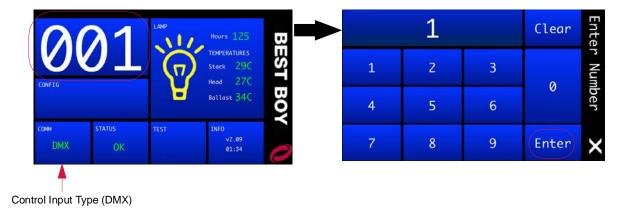
Figure 2-15: Setting Starting Address (DMX Control)
