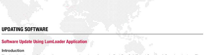
The LumLoader application allows you to update the software in Bad Boy® (HP and Standard) Spot Luminaires. The update will be sent over an Ethernet connection. The luminaire can take the Ethernet input directly, or the update can be translated to DMX512 signal with an appropriate device, either Series 400® or a PRG Node. The fixtures can be daisy-chained to load multiple fixtures at once.
