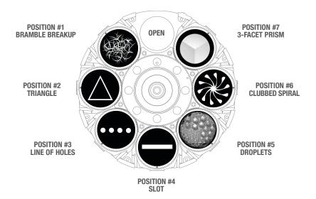
The following charts represent the standard gobo wheel configurations for the Bad Boy CMY<sup>®</sup> Spot luminaire.
